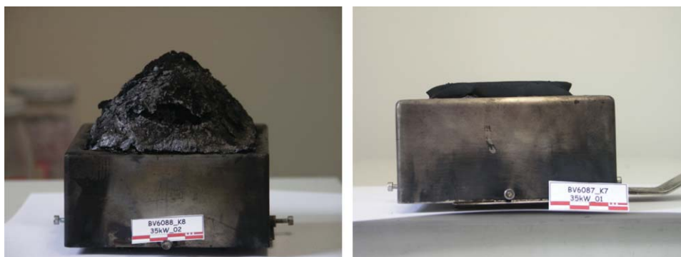
Figure 7 Fire residue of EP+15 wt % APP (on left) and EP+LS+10 wt % APP (on right). Combining APP with LS influences the intumescence and quantity of the char. The illustrated inhibition of intumescence is concluded to cause the antagonism in EP+LS+10 wt % APP. [Color figure can be viewed in the online issue, which is available at www.interscience.wiley.com .]
